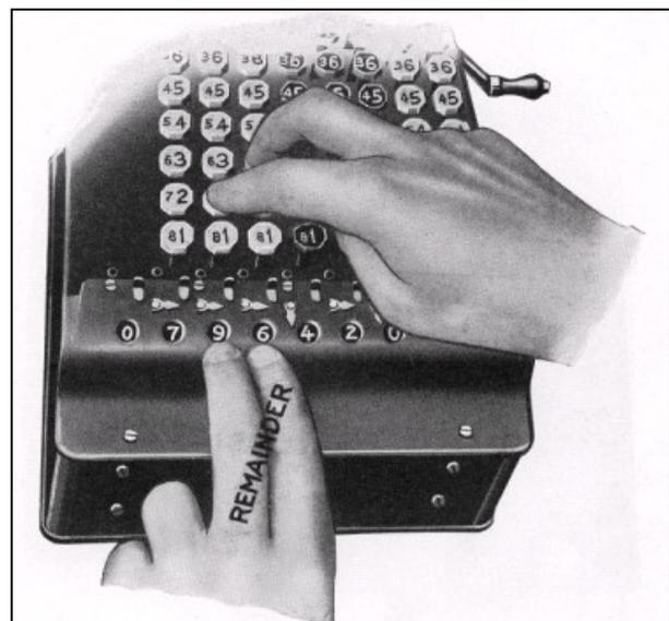
Press these keys representing the divisor repeatedly while counting the strokes out loud until the number of strokes made agrees with the figure standing in the register in the next column to the left of those on which the keys are being struck. See cut on opposite page where this figure is a "6" and is marked "Index."
